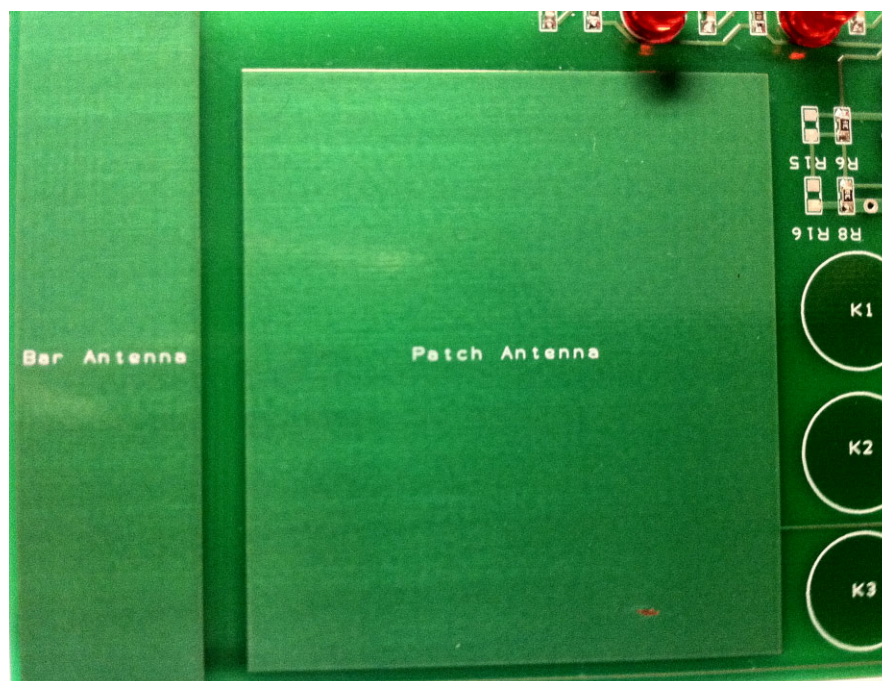
Figure 4-1. Examples of a Bar and Patch Sensor Implemented on a PCB
